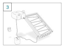
We don't need the rack for the explanation, so we'll hide it. The input tank is connected with the absorber through a tube (or pipe). In the middle, hidden behind the output tank, there is the insulated riser, from which the treated water will flow into the output tank.
