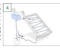
First of all, the input tank is filled with the water that should be treated. Via the tube the water level in the absorber rises to the same fill height as the input tank.
