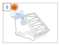
At the end of the day the all of the water in the output tank got treated. If the sun is not strong enough to treat all the water there will be water left in the input tank.
