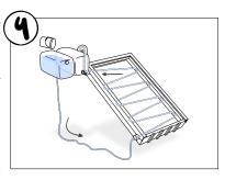
The sun heats the water in absorber. A good insulation is very important.
